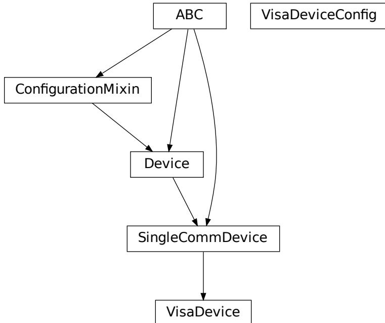
**class VisaDevice**(*com*: VisaCommunication | VisaCommunicationConfig | *dict*, *dev\_config*: VisaDeviceConfig | *dict* | *None* = *None*)
