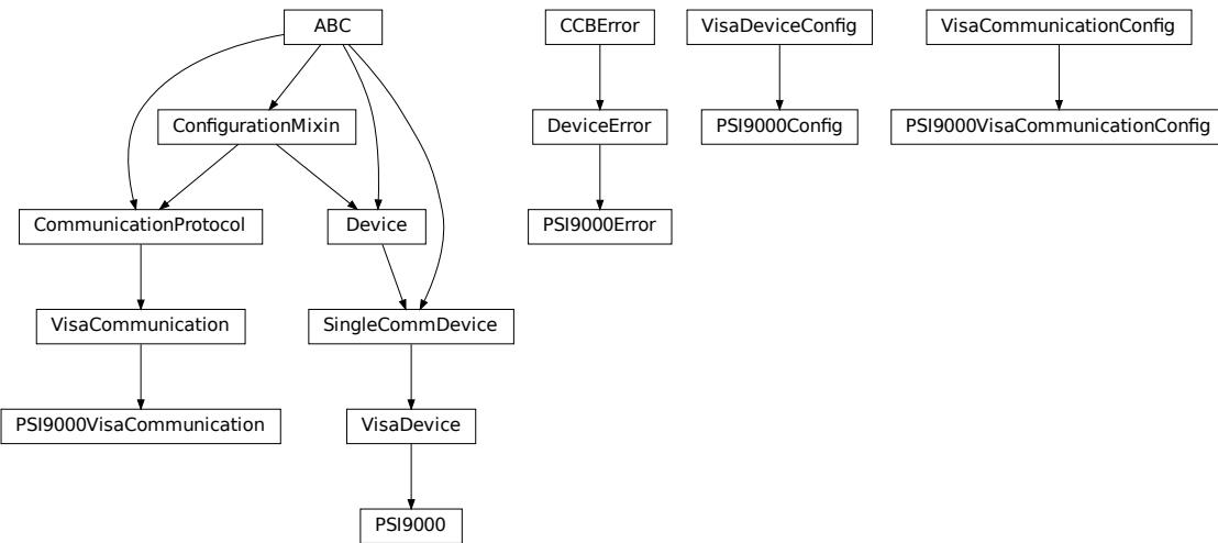
Device class for controlling a Elektro Automatik PSI 9000 power supply over VISA.
