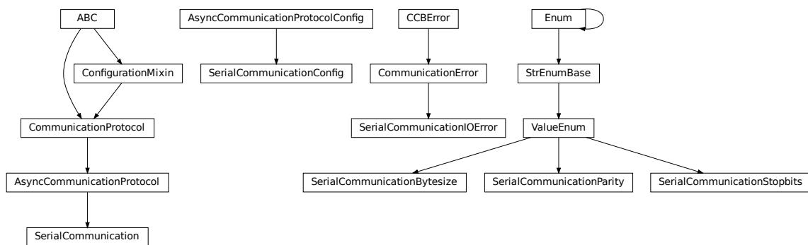
Communication protocol for serial ports. Makes use of the `pySerial` library.
