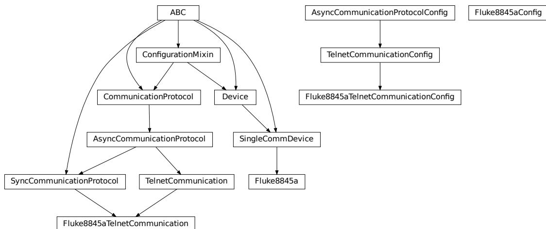
Python module for the Fluke8845a Multimeter. The communication to the device is through Telnet. 8845A/8846A Programmers Manual is available in the following link. All page numbers mentioned in this script refer to this manual. [https://download.flukecal.com/pub/literature/8845A\\_pmeng0300.pdf](https://download.flukecal.com/pub/literature/8845A_pmeng0300.pdf)
