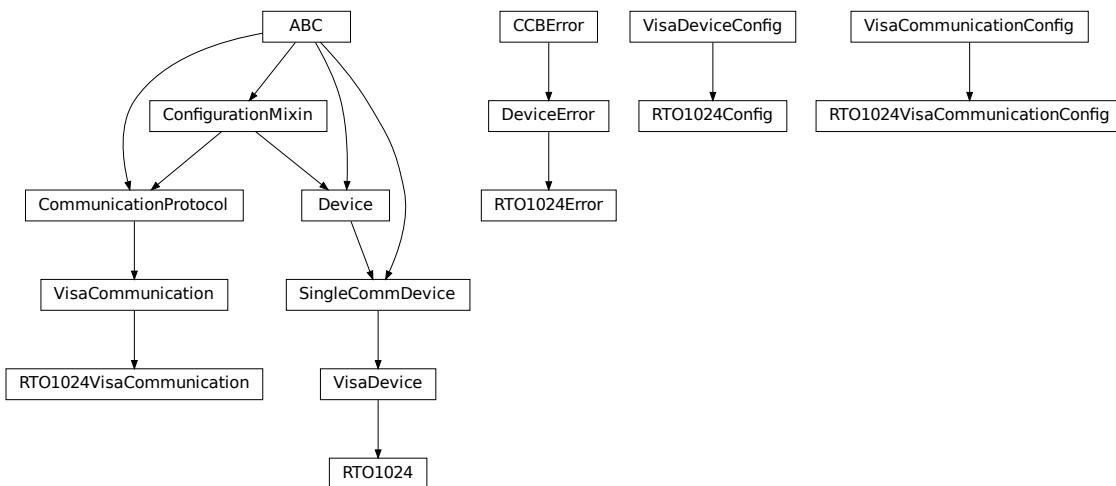
Python module for the Rhode & Schwarz RTO 1024 oscilloscope. The communication to the device is through VISA, type TCPIP / INSTR.
