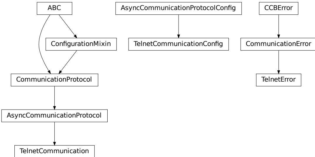
Communication protocol for telnet. Makes use of the `telnetlib` library.
