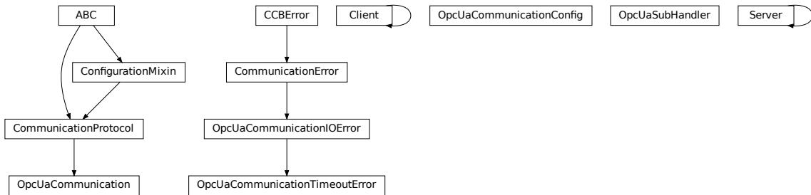
Communication protocol implementing an OPC UA connection. This protocol is used to interface with the “Cube” PLC from Siemens.
